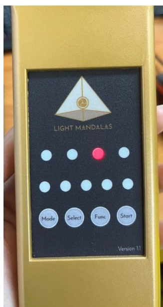
Mandala Wand Screen – 3 rd Red light shows user is using Bluetooth Mode
