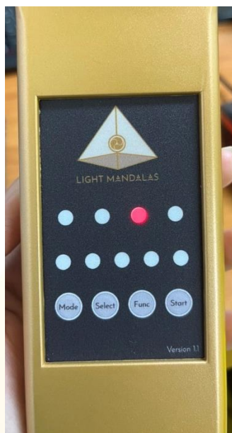
Mandala Wand Screen – 3 rd Red light shows user is using Bluetooth Mode
